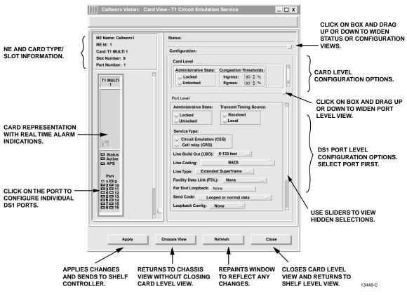
Figure 755-1. T1 Multi 1 Card Configuration Window
